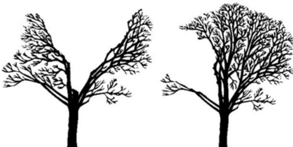
Figure 36. Example of trees directionally pruned for clearance from power lines
